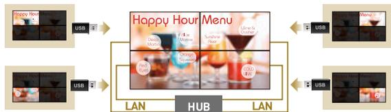
Connecting more than one unit with LAN cable reproduces files in USB memory simultaneously. One of the units becomes Master, and the others Slaves.
