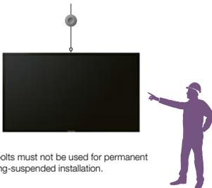
\* Eyebolts must not be used for permanent ceiling-suspended installation.
